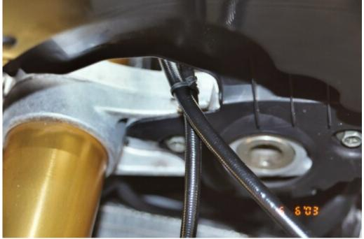
Left line and right line must cross as seen in picture, as this allows for line to MOVE and FLEX at the correct spots. This positioning is VERY IMPORTANT (allows for fender clearance)!
