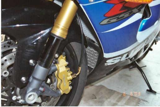
G) Brake lines under lower triple clamp, READ BELOW!!!
