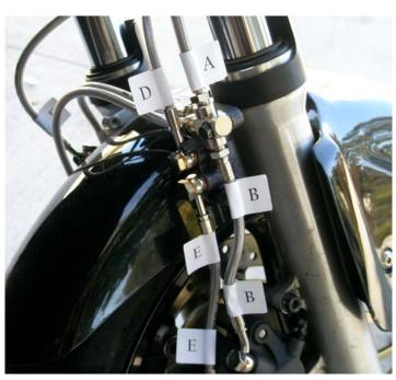
c. Lines A, B, D & E at right caliper delay valve
