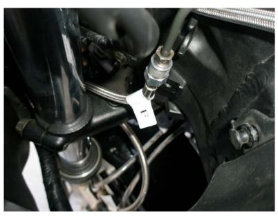
r. Line F routed in front of the lower triple tree
