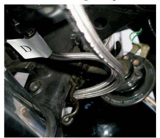
g. Lines A & D routing in front of the lower triple tree
