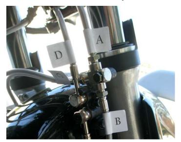
d. Lines A & B t-block and Line D at right caliper delay valve
