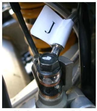
v. Line J at rear master cylinder with OEM tubing and bolt
