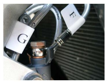
l. Line F installed at left caliper secondary master cylinder Line G routed behind
