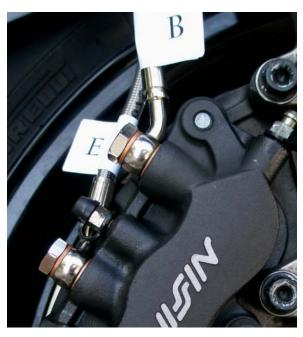
j. Lines B & E installed to right caliper
