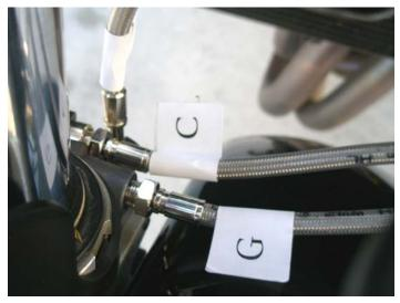
k. Lines C & G crossover lines at right caliper delay valve
