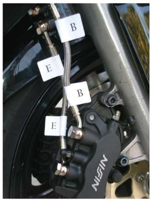
e. Lines B & E from delay valve to right caliper
