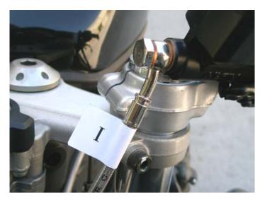
s. Line I at clutch master cylinder
