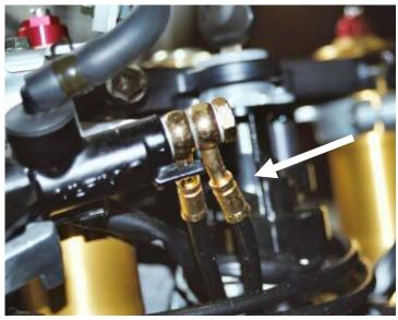
A. Master Cylinder (Note: the left line is positioned slightly in front of the right line)
