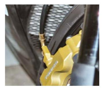
D. Note: the position of the brake line is slightly away from the bike
