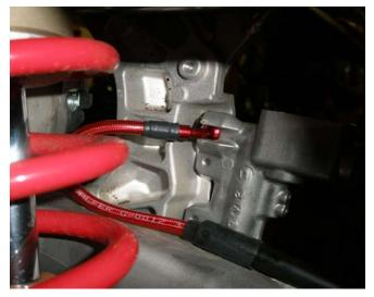
B. Rear Master Cylinder (re-attached to frame)
