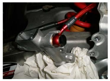
A. Rear Master Cylinder (removed from frame)
