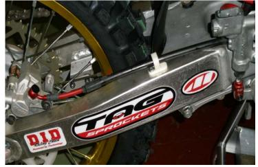
C. Line routed down the swing arm to caliper
