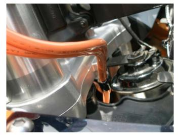
c. Routing at lower triple tree
