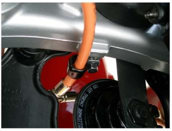
b. Top line routed through the Galfer c-clip at lower triple tree
