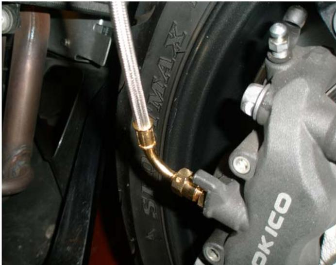
**C. Right Caliper, notice the line is slightly away from the bike**
