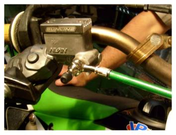
A. Master Cylinder (with optional Galfer bleeder bolt)
