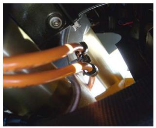
c. Galfer c-clips at lower triple tree
