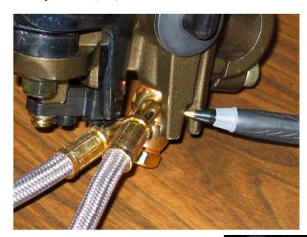
Master Cylinder Modification Picture to the left: Front master cylinder removed from bike, Galfer lines installed and pen indicating which tab to grind off
