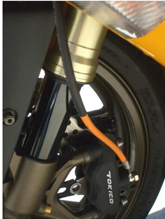
**d. Left caliper, Galfer line routed in front of fork, notice fitting position**
