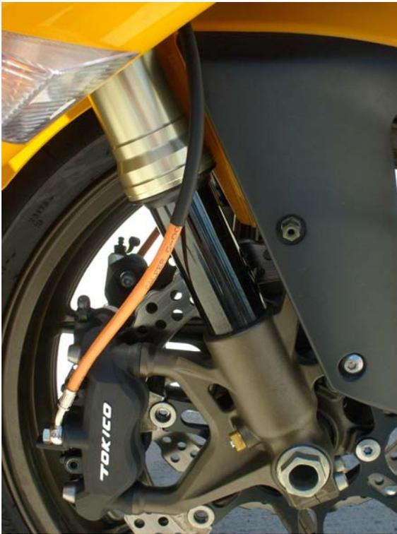
**c. Right caliper, Galfer line routed in front of fork, notice fitting position**
