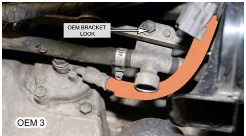
(Fig: OEM3) Remove mounting bolt/coolant drain valve, pull forward and up to access slave cylinder.
