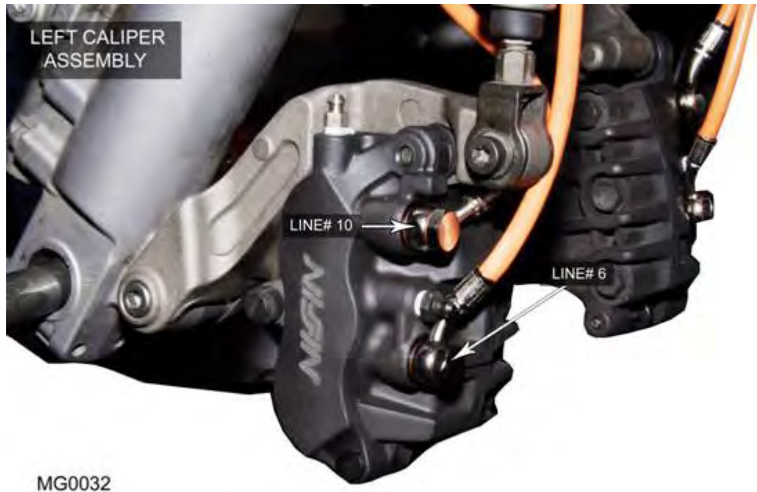
(Fig: MG0032) Left caliper is shown with Line# 6 connected to bottom hole from Galfer's T-block (MG0025) see ref. Line# 10 is connected to upper hole from the backside of the 2 nd Master Cylinder.
