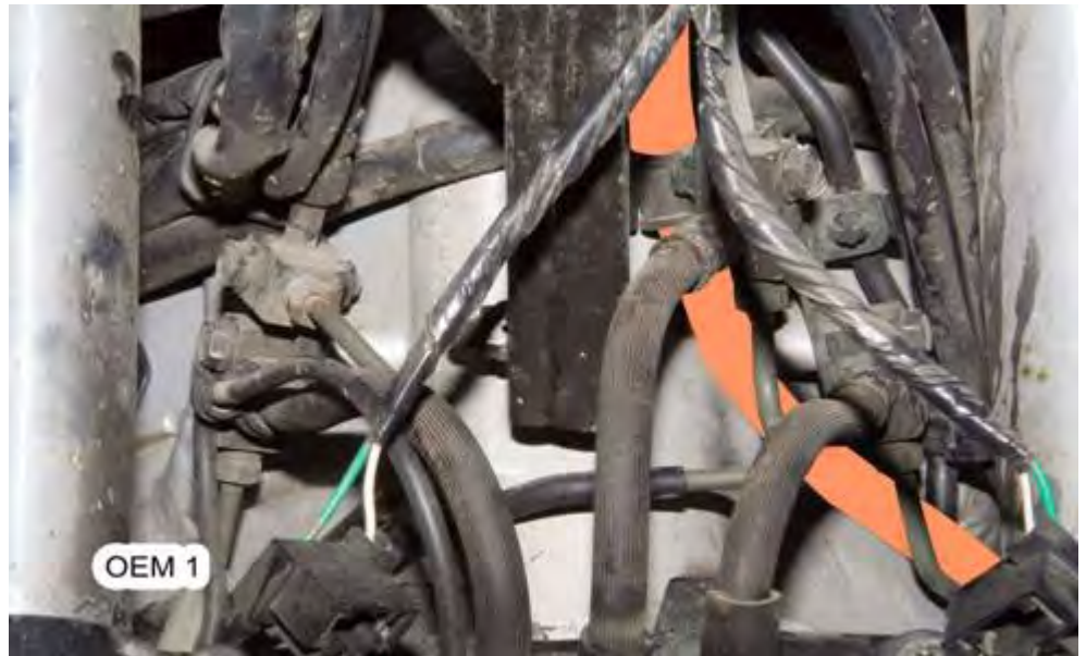
(Fig: OEM1) Following stock routing under left handle bar cover, across top triple clamp retainer
