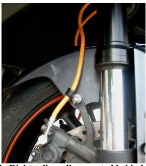
b. Right caliper, lines routed behind forks and Galfer c-clip at fender
