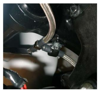
**B.** Left Line of the T-block secured by the Galfer C-Clip at Triple Tree
