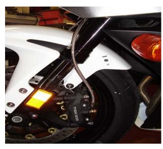
E. Line Routed in Front of the Fork to the Left Caliper
