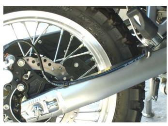
b. Galfer line routed down swing arm, notice OEM clip by the master and the Galfer provided c-clip by the caliper
