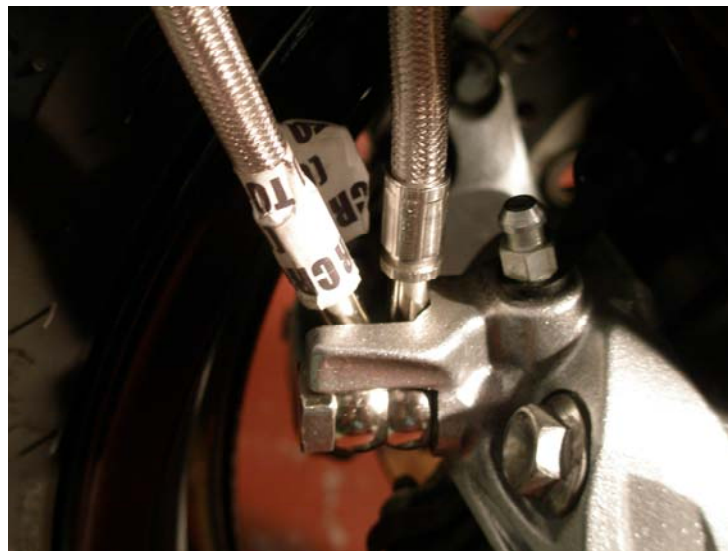
C. Right Caliper with Master Cylinder line and Crossover Line installed
