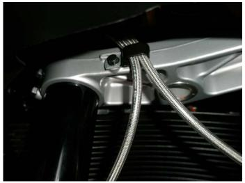
b. Galfer c-clip at lower triple tree, lines routed behind the forks
