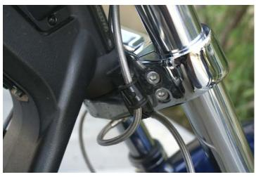
b. OEM line holder at the lower triple tree
