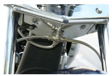
c. Galfer t-block at the lower triple tree
