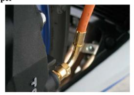
e. Left caliper, notice position of fitting
