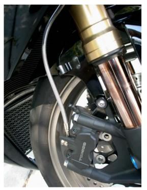
f. Right caliper routing
