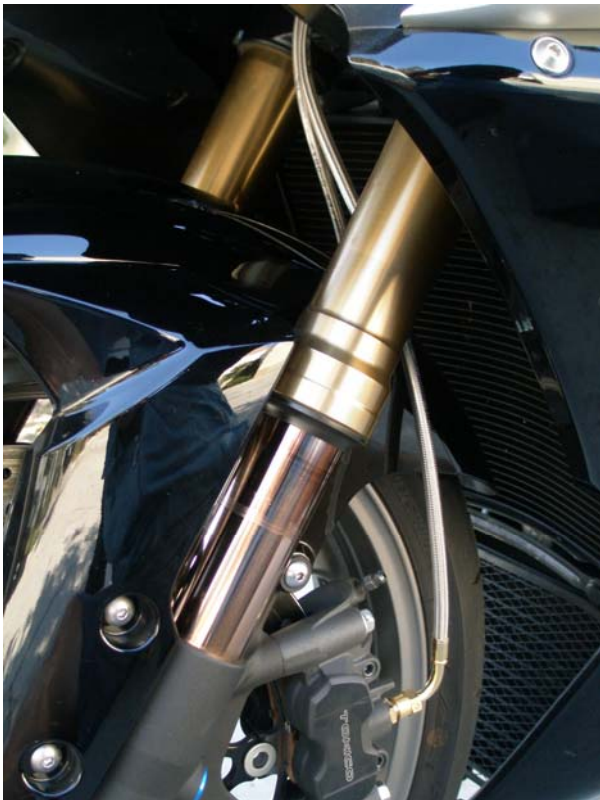
c. Left caliper, with lines routed the behind forks
