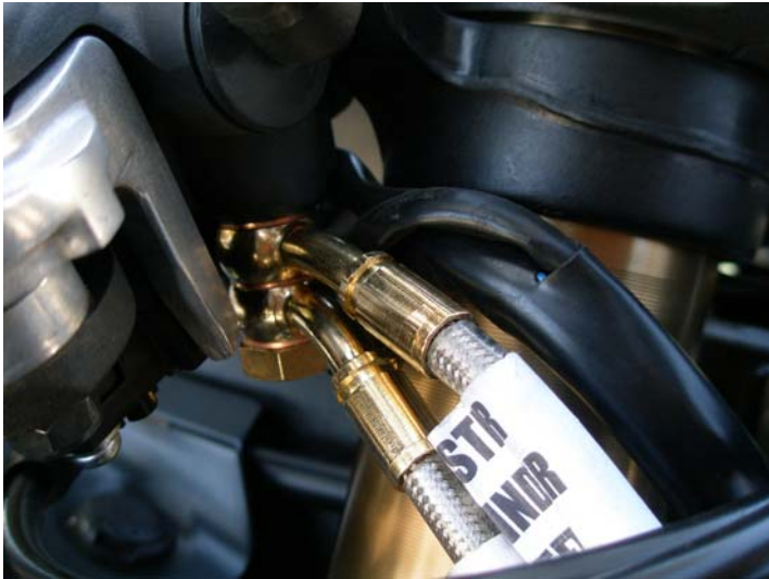
a. Front master cylinder, notice positioning of fittings
