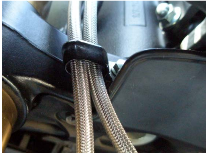
b. Galfer c-clip at lower triple tree
