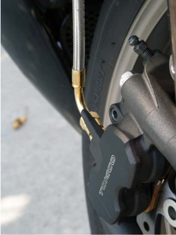
f. Right caliper, notice fitting is pointing away from bike a bit
