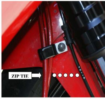
F. Lines C & B at Galfer C-Clip on Right side of fender
