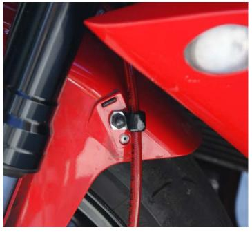
G. Line B at Galfer C-Clip on Left side of fender
