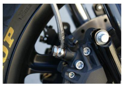
e. Banjo installed at front caliper, using washer, banjo, washer, bolt sequence
