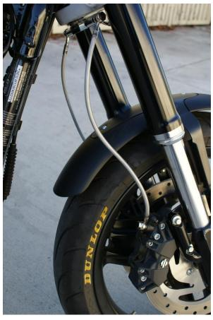
f. Right and left line routing from union to calipers
