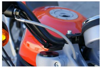
a. Front master cylinder, line A routed through the upper triple tree
