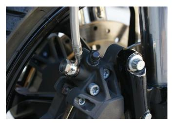
D. Banjo fitting, with bolt and washers, installed on caliper
