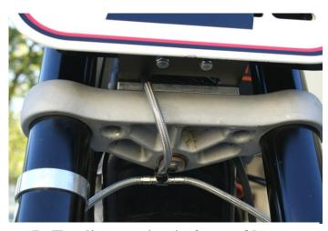
B. Top line routing in front of lower triple tree, Galfer c-clip replacing union
