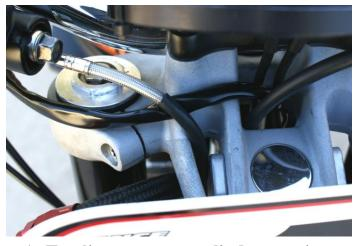
A. Top line at master cylinder, routing through upper triple tree
