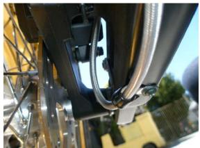
e. Routing from c-clip; behind the swing arm to the rear caliper
