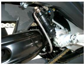
a. Rear master cylinder and routing underneath bike
