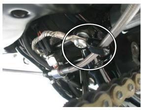
b. Brake light switch from master cylinder, Galfer larger c-clip in circle
