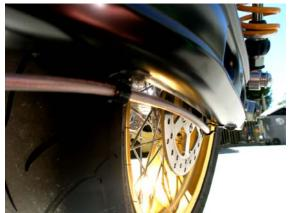
d. Swing arm routing, Galfer c-clips replacing stock
