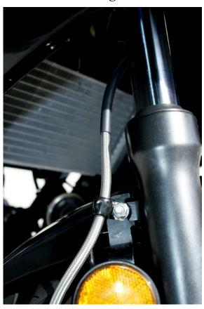
c. Galfer c-clip at fender, routing behind fork
