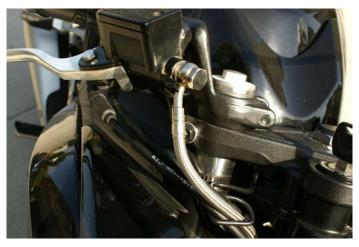
a. Front master cylinder, notice the routing
