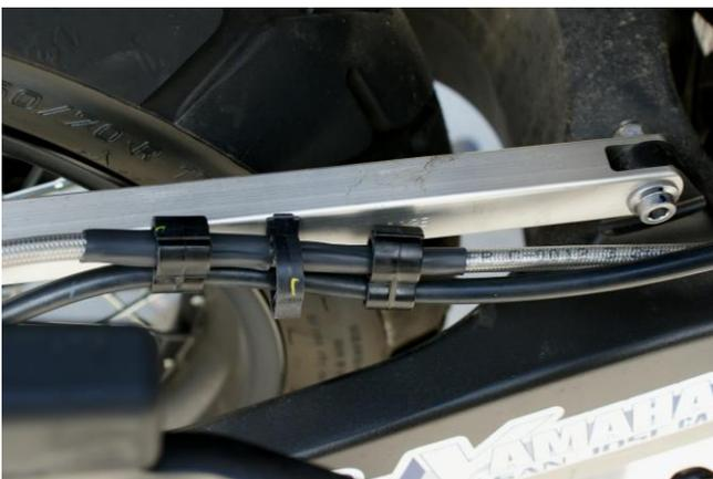
**Line I – OEM routing at Swing Arm, notice lines crossing**
