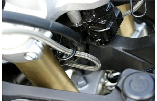
**Line A – Routing from Master Cylinder**
