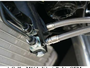
j. Galfer M16 bolt installed to OEM bracket at the lower triple tree
