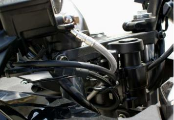
a. Line A installed to front master cylinder
