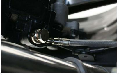
n. Line E installed at rear caliper GALFER USA
