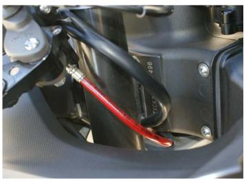
**B.** Master Cylinder Line Routing
