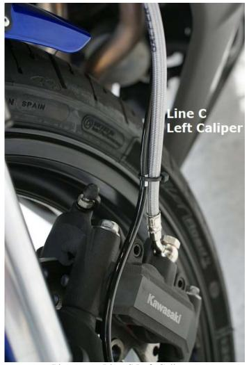
Picture 6 – Line C Left Caliper
