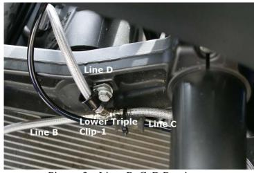
Picture 3 – Lines B, C, D Routing
