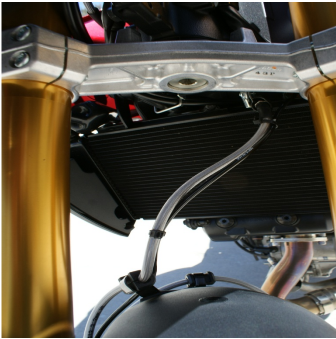
Line-B reusing OEM grommets / routing with 3 zip ties Picture-3
