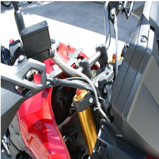
Line-A using OEM routing ring Picture-1
