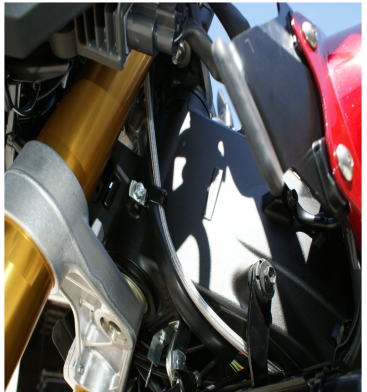
Line-D OEM routing with CLIP-2 provided Picture-8
