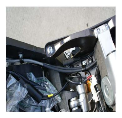
Line-A-D right frame routing to ABS Unit
