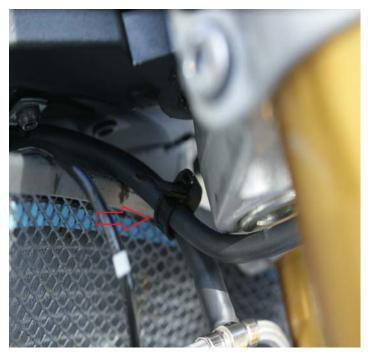
Rear caliper / rear master cylinder Line-E-F Routing Using Clip-2 bottom tail section Using the provided M6 bolt and Nut
