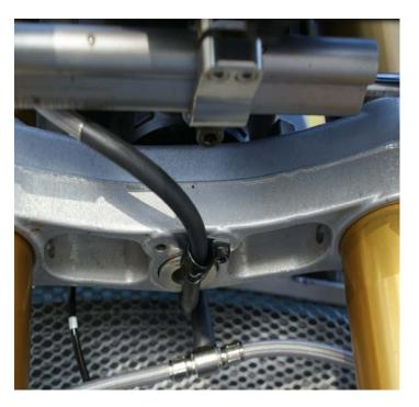
Line-A routing lower triple using
