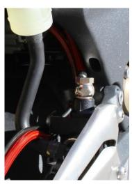
Make sure to tighten the rectifier bracket bolts once you are done routing the lines, as well as reattach the wiring harnesses. Double check clearance of the new lines under the tank, and verify all vacuum tubing, wiring harnesses, airbox, and mounting bolts are in place before proceeding.
