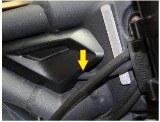
Continue running the line rearward along the right frame rail, through the 3 factory clips, and to the *right-forward* port on the ABS unit.
