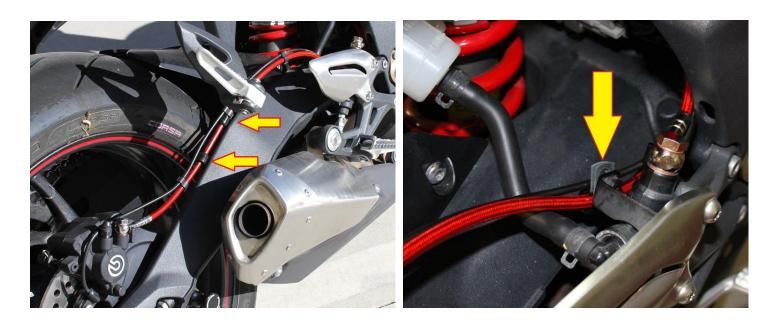
Route the line forward and behind the rectifier. It will attach to the OEM clip on the back side of the bracket. Route the line up to the *left-rearward* port on the ABS unit and attach.
