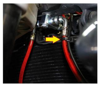
Run the lines to their respective calipers and install with the provided bolts and crush washers. Use the last provided zip tie to attach the ABS sensor wire to the left line. The line should also be run through the bleeder cap.
