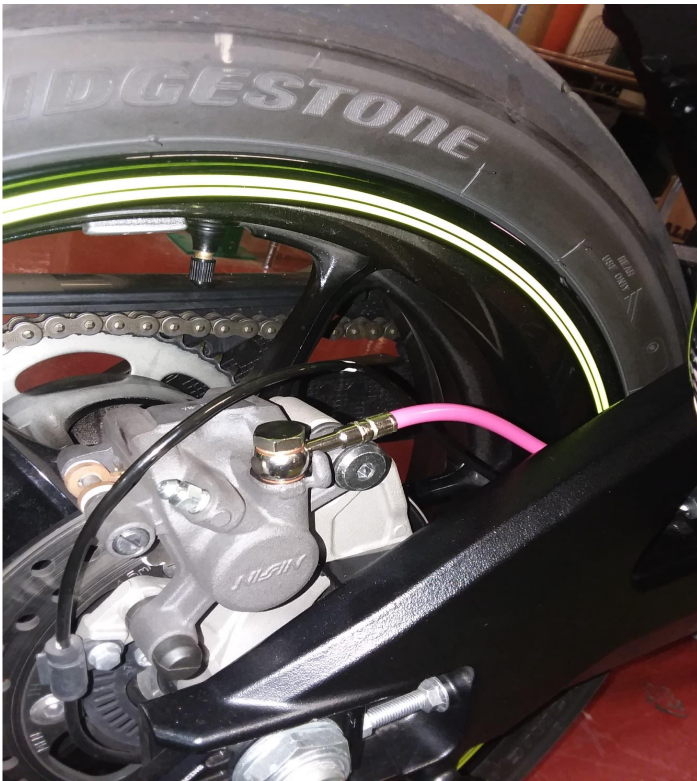
(PICTURE F) CONTINUED, BANJO INSTALLED ONTO CALIPER
