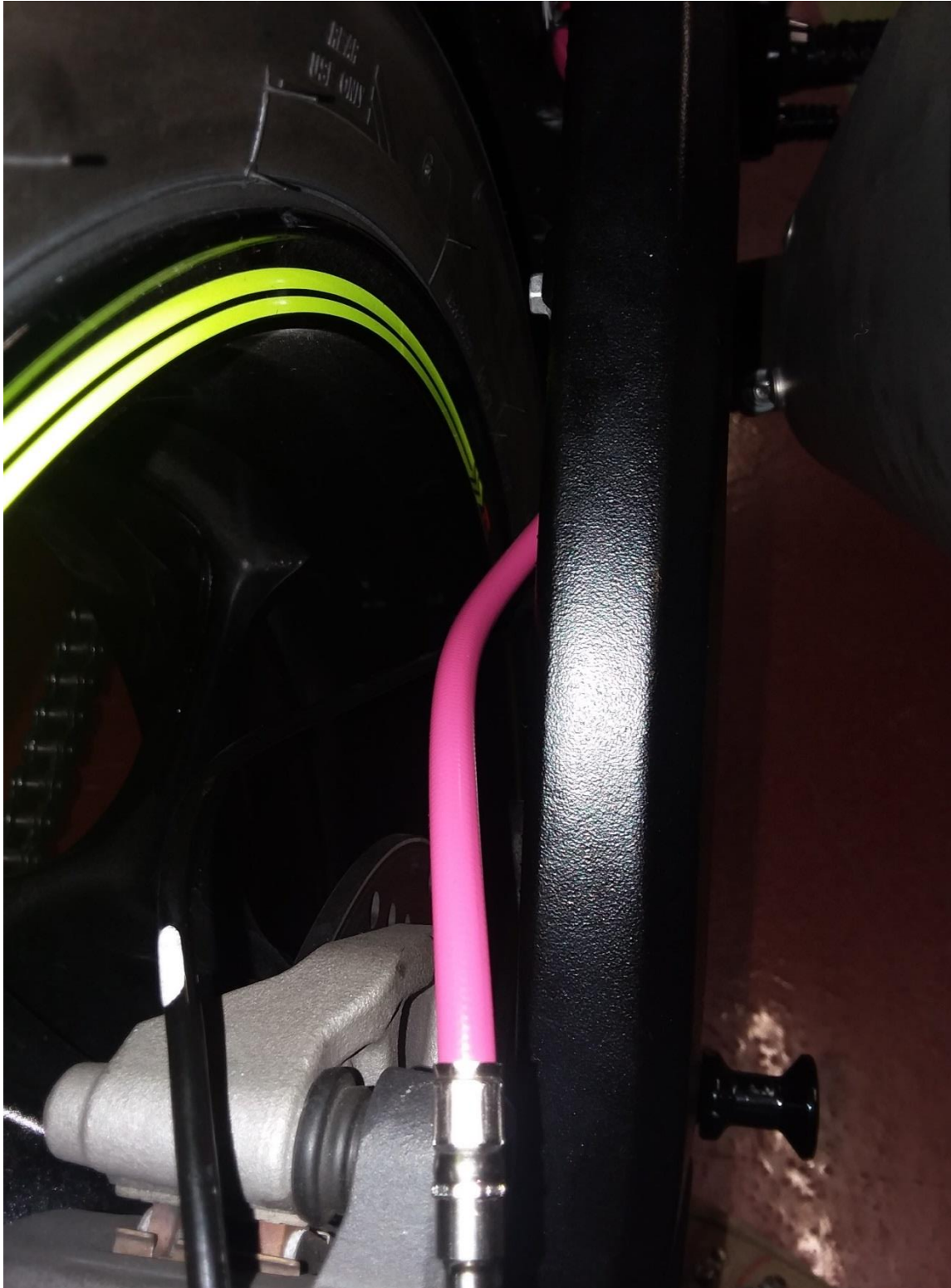
(PICTURE F) FACTORY ROUTING AROUND SWING ARM
