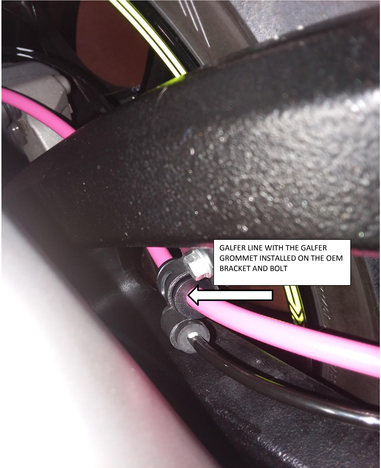
(PICTURE E) O.E.M HOLDER/BOLT WITH GALFER GROMMET
