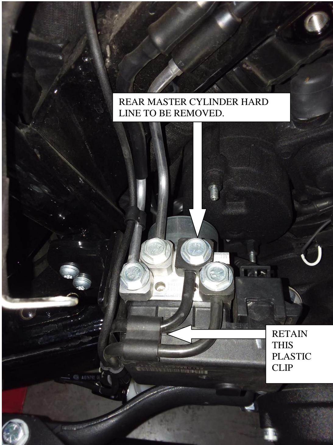
FIGURE 4 A.B.S. REAR LINE LOCATION
