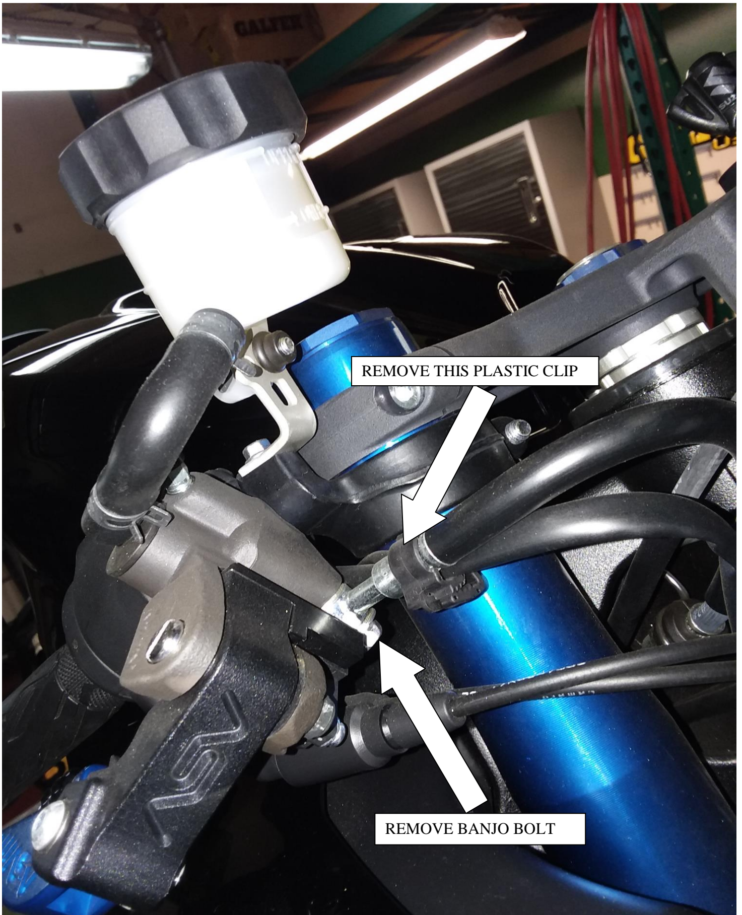
FIGURE 3: BOLT AND PLASTIC CLIP
