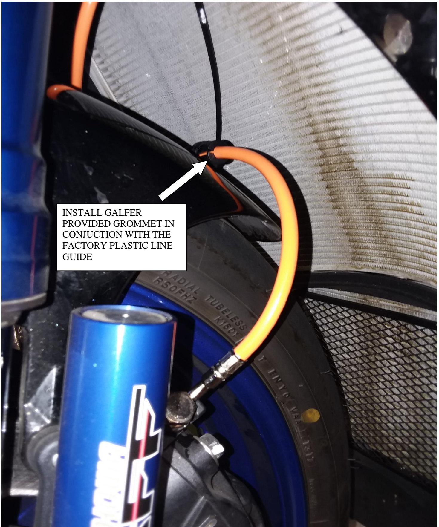
FIGURE 16: LINE HOLDER/GROMMET & LEFT CALIPER
