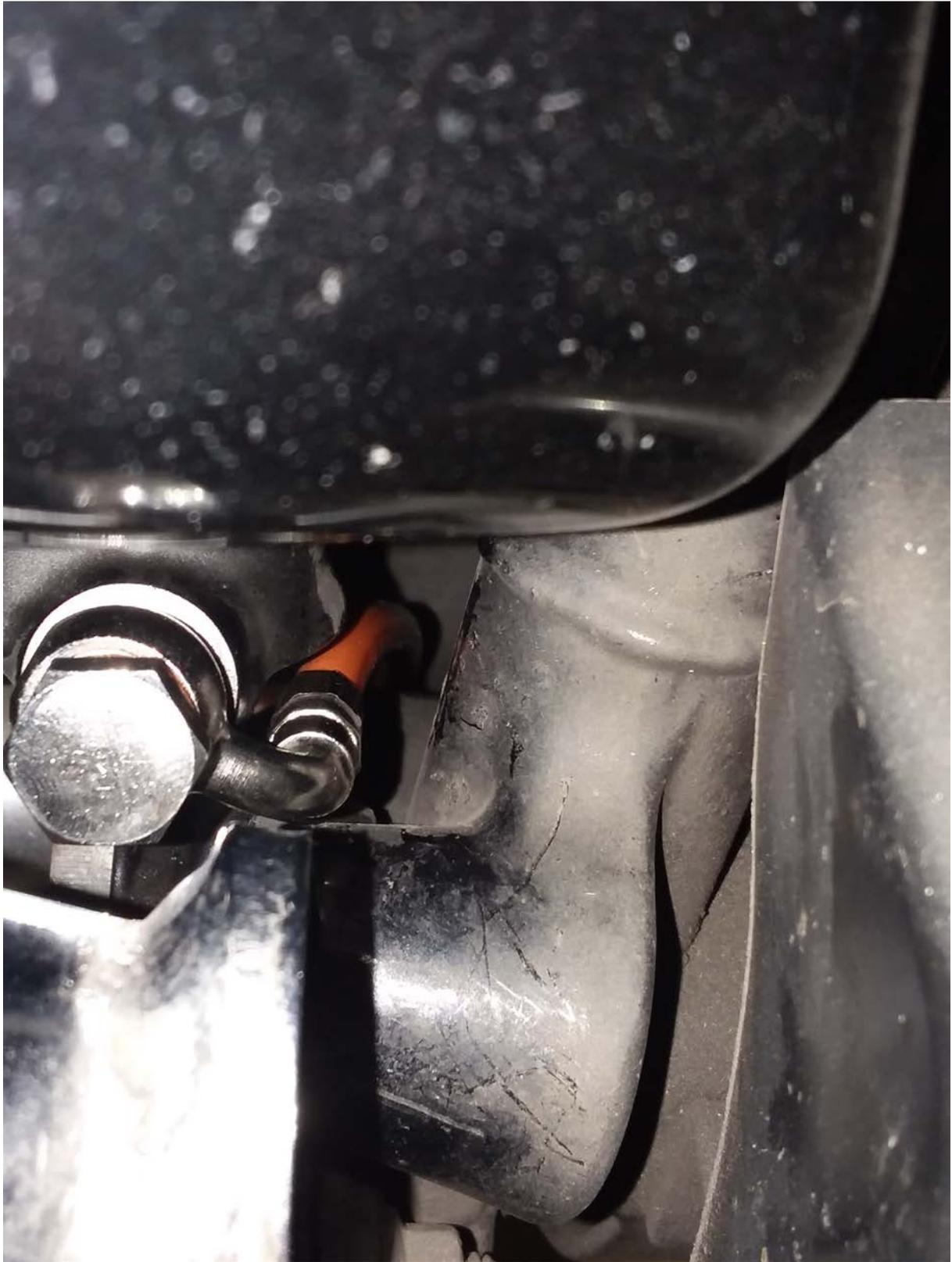
**FIGURE 16 LINE E INSTALLED ONTO MASTER CYLINDER**
