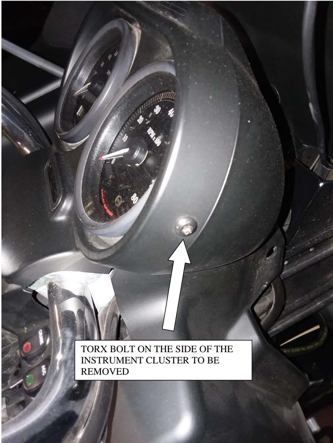
TORX BOLT ON THE SIDE OF THE INSTRUMENT CLUSTER TO BE REMOVED
