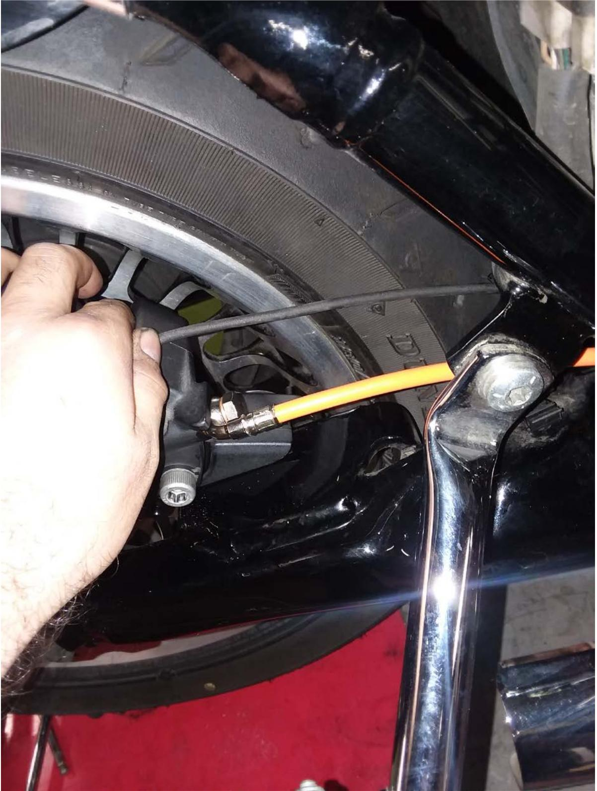
**FIGURE 21 CONTINUED CALIPER INSTALL**
