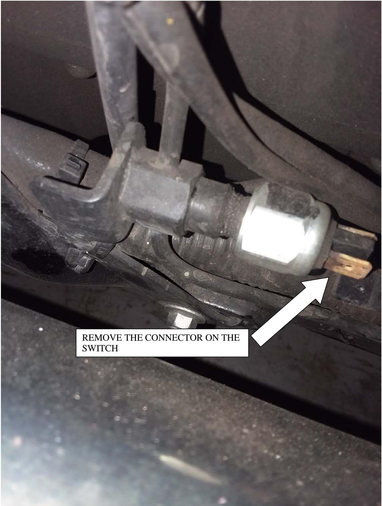
REMOVE THE CONNECTOR ON THE SWITCH
