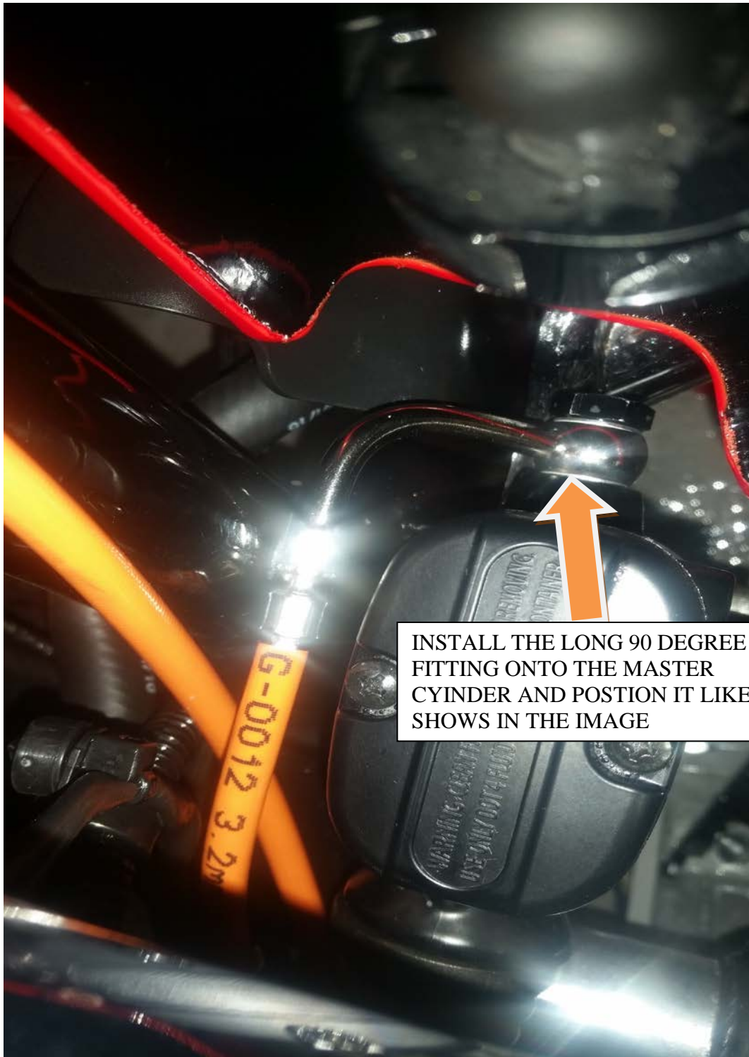
FIGURE 21: REAR BRAKE MASTER CYLINDER
