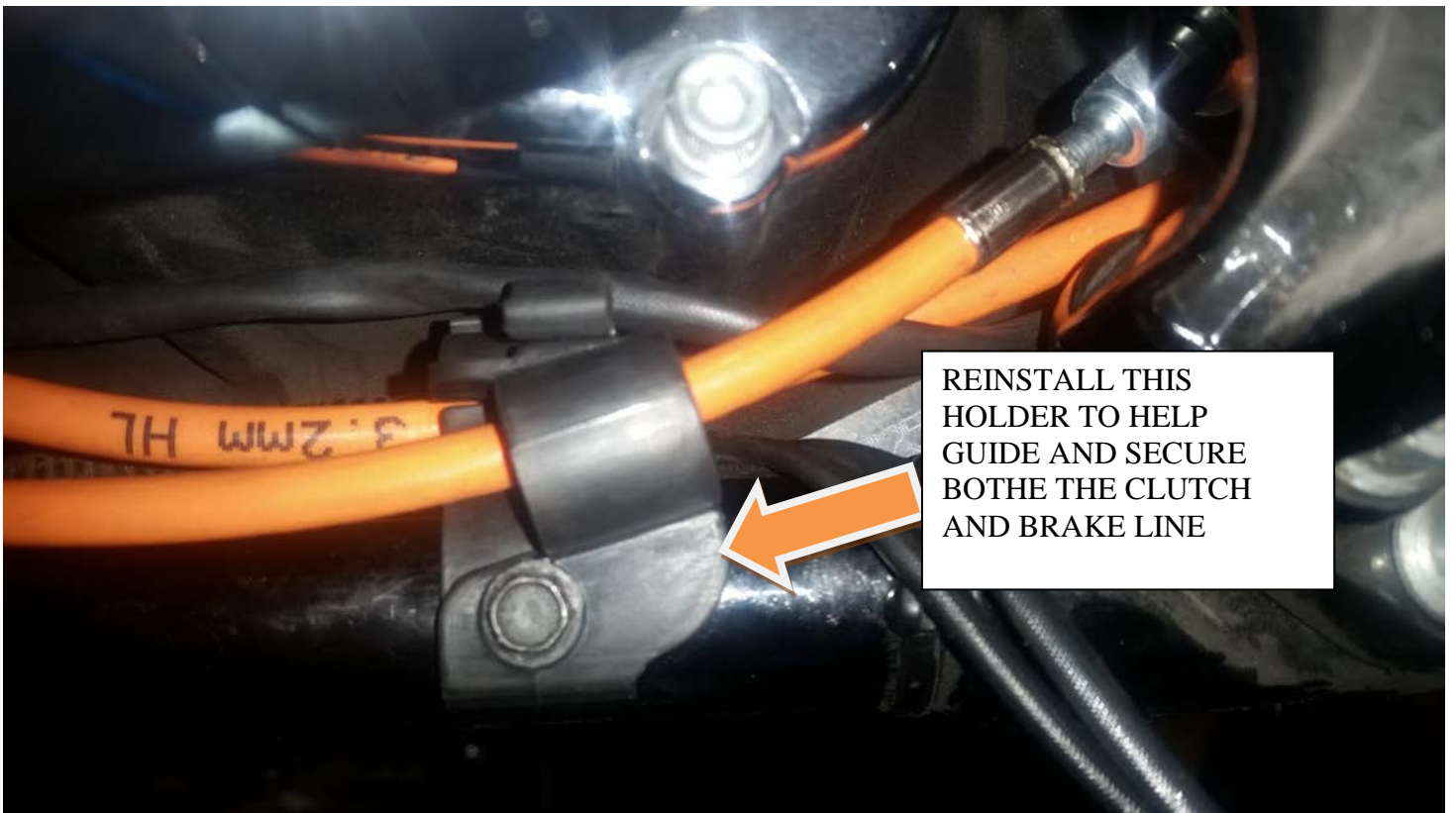
FIGURE 28: LINE HOLDER CLUTCH/BRAKE
