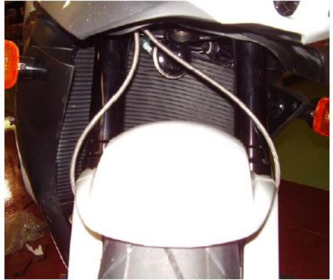
B. Overall Line Routing
